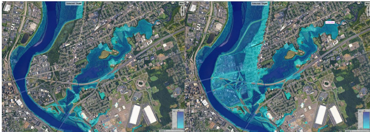
Figure 32. Projected Flooding at East Hartford Breach Location BL2 for the Top of Levee Loading Scenario for Non-Breach (Left) and Breach (Right) Conditions
