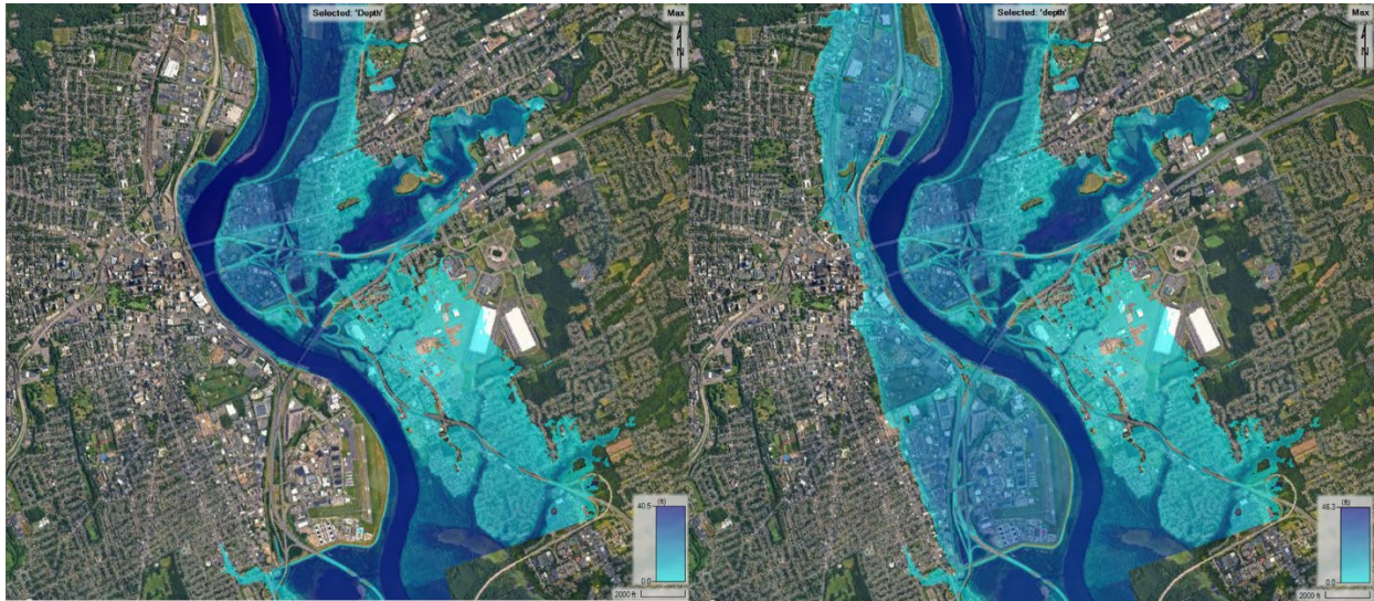
Figure 29. Projected Flooding at Hartford Breach Location BL2 at the Top of Levee Loading Scenario for Non-Breach (Left) and Breach (Right) Conditions
