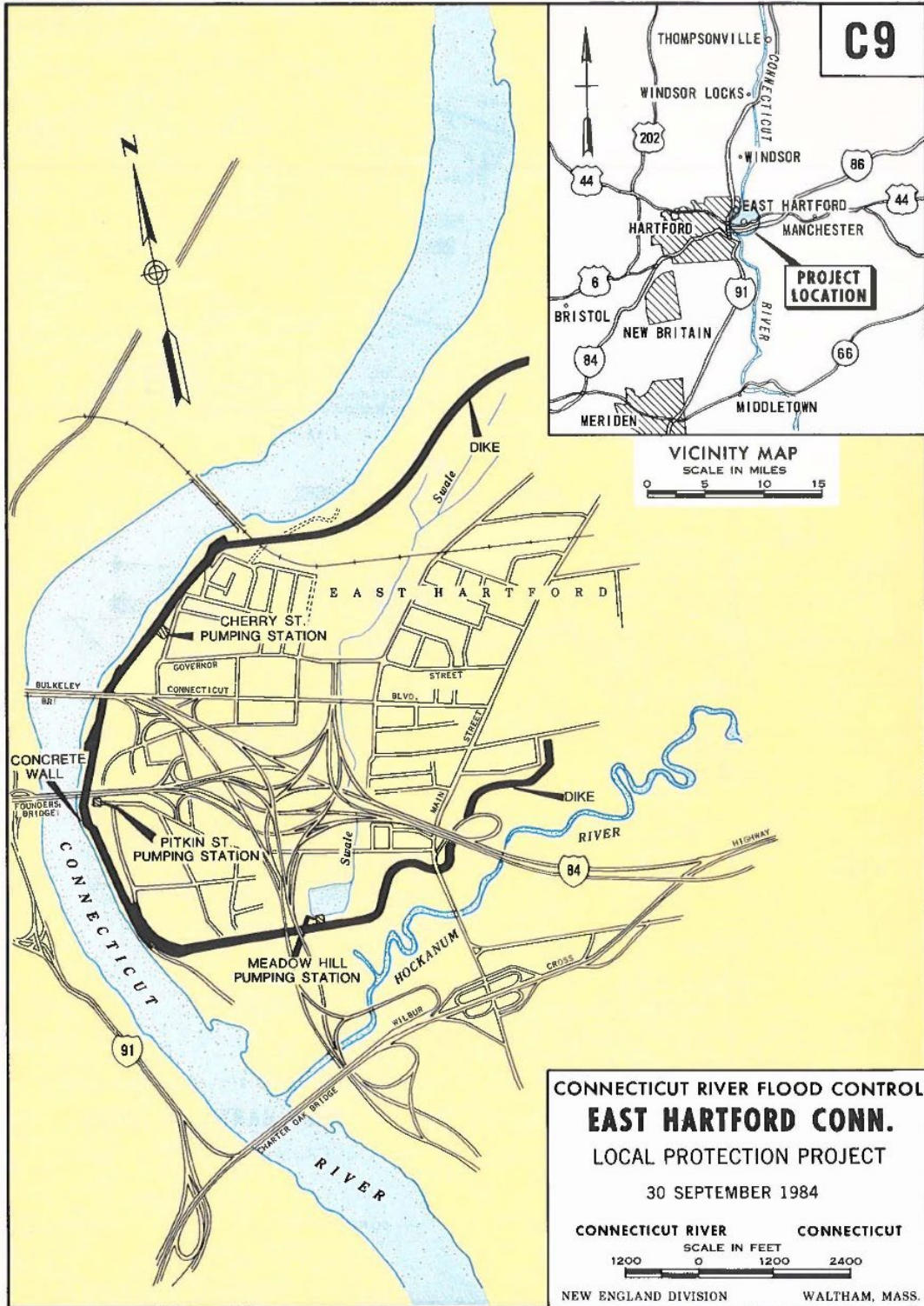
Figure 9: The East Hartford Flood Risk Management System
