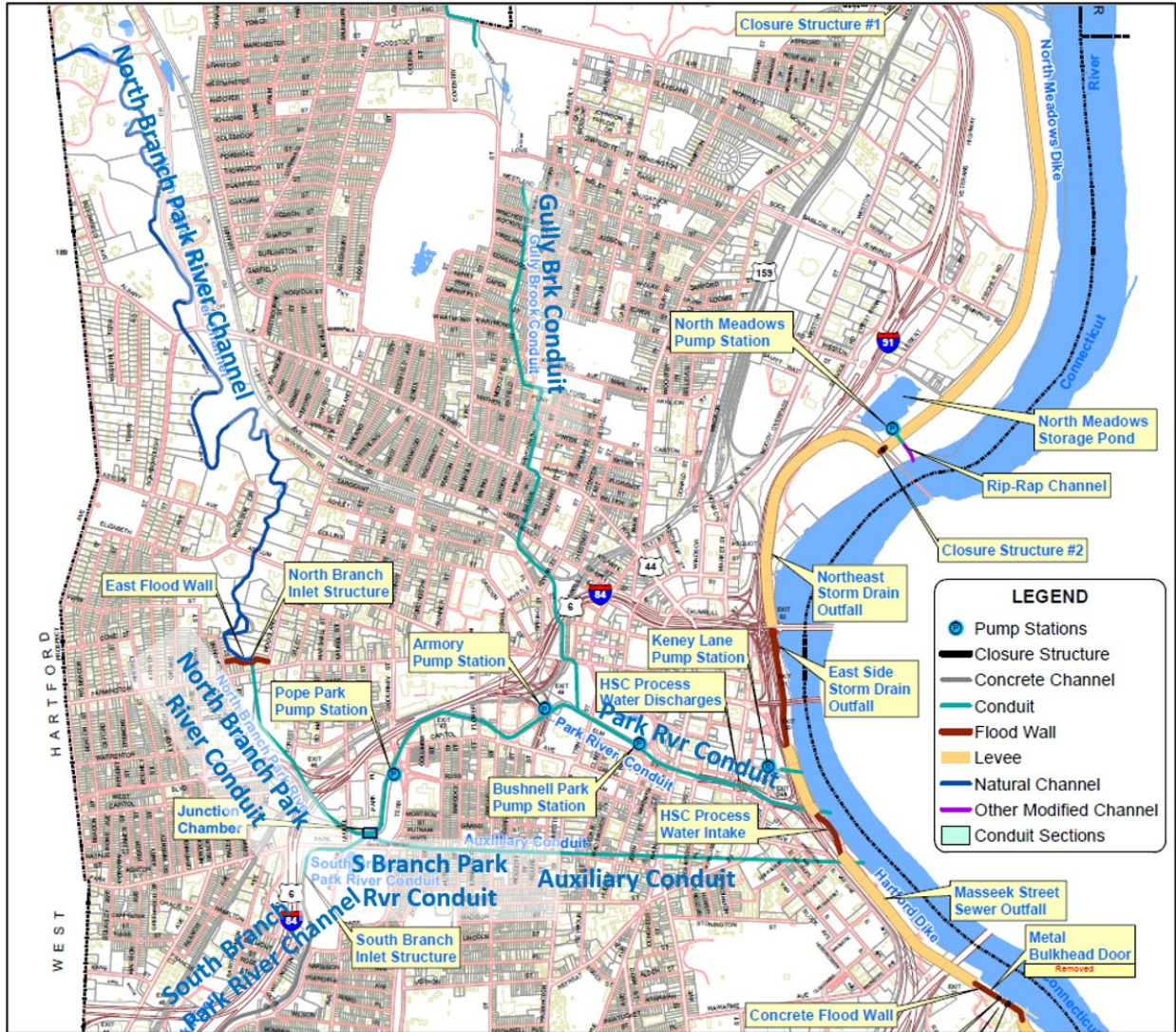
Figure 7: Gully Brook, North and South Branch Park River, Park River, and Auxiliary Conduits in the Northern Hartford Flood Risk Management System
