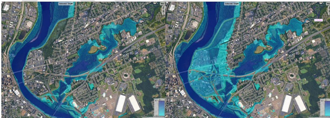
Figure 33: Projected Flooding at East Hartford Breach Location BL3 for the Top of Levee Loading Scenario for Non-Breach (Left) and Breach (Right) Conditions
